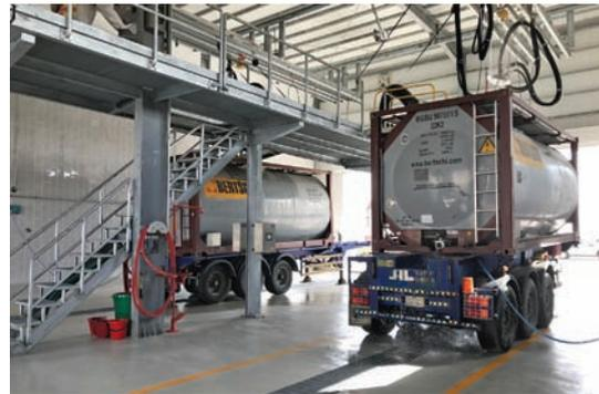
*The facility has two washing lines with four washing bays for tank containers or two washing bays for road tankers. We can clean most hazardous goods and offer 2½- and 5-year inspections and other repair and maintenance work* Andreas Nebiker, Aldrees Bertschi terminal, Saudi Arabia
